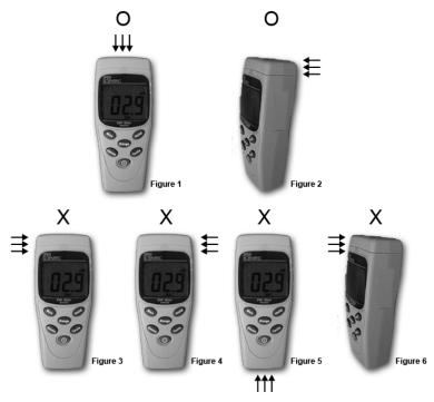
Arrow pointing direction indicates the direction of electromagnetic waves.
