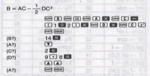
Since the SOLVE function uses Newton's Method, certain initial values (assumed values) can make it impossible to obtain solutions. In this case, try inputting another value that you assume to be near the solution and perform the calculation again.
