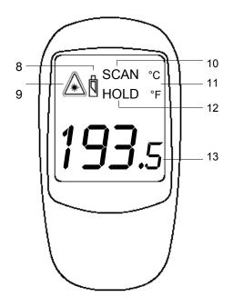
8. Low Battery Indicator 11. °C & °F9. Laser Guide On/Off 12. Hold
